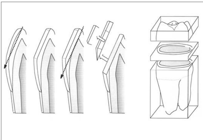
**Fig 2** Localization and preparation technique for enamel and dentin sections of natural teeth used for colorimetric and opacity measurements (each type of section is  $1.0 \pm 0.05$  mm).
